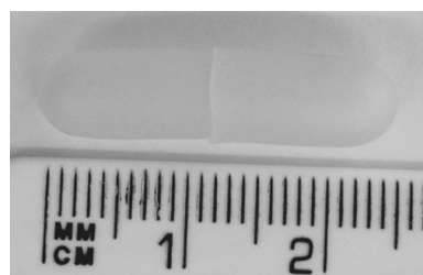
Figure 1 Capsule formed using formulation 5 (17% HPMC, 0.2% gellan gum, 2% sodium alginate)
