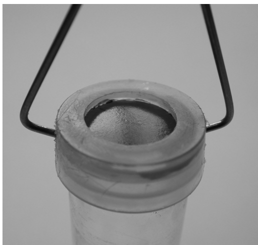
Figure 3 Dissolution vial used for enteric film experiments showing polymer film (dyed with brilliant blue) surface to be exposed to the dissolution medium
